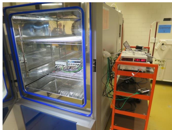
Overview climate chamber and measuring instruments
